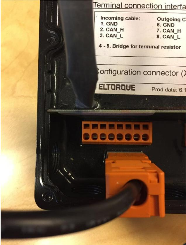
Figure 5 Eltorque Configuration Cable connected to port
