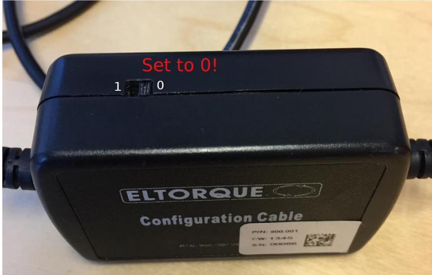
Figure 4 Eltorque Configuration Cable and switch
